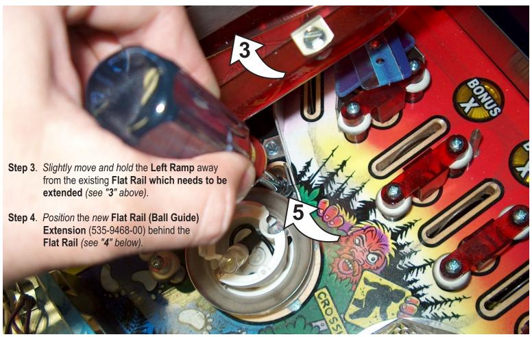
Step 5. Fasten the new Flat Rail Extension to the playfield with the enclosed #8 X 1/2" HWH Screw (see "5" above).
